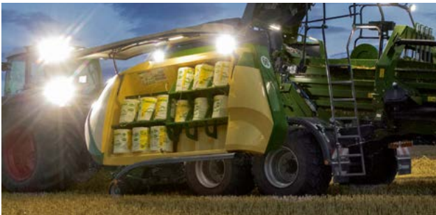
Lights inside the twine boxes
