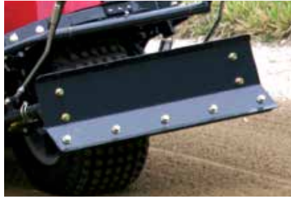
The front blade option smooths and evens the bunker.
