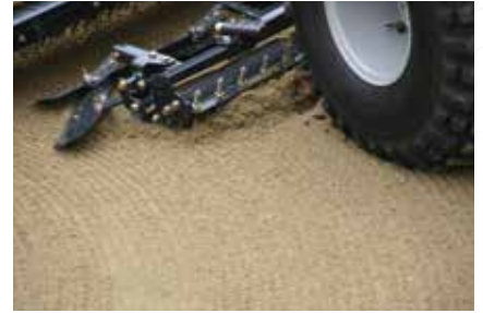
The cultivator option breaks up and softens coarse sand.
